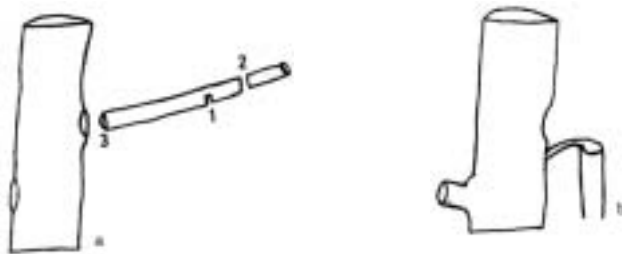
Figure 4. Proper (a) and improper (b) ways to make a large cut. First cut 2/3 through the bottom of the limb (1) about two feet from the trunk. Next completely saw through the limb at (2). Lastly, remove the branch flush with the trunk (3) leaving no stub.
